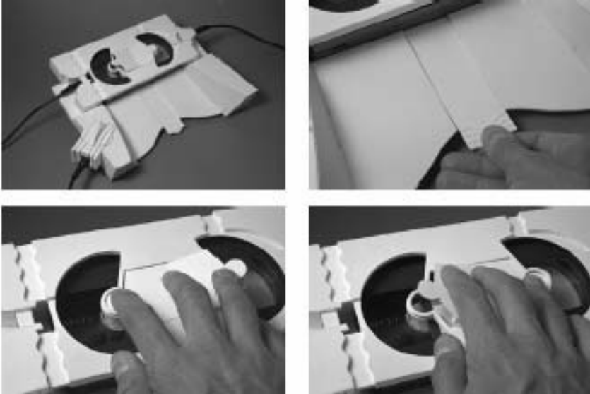
Figure 2. The action of the user opens up the functionality. Starting top-left clockwise: the cassette remains visible whilst in the machine, pulling a ribbon triggers eject, and fast-forward/reverse becomes intuitively clear through a toggle placed between the tape reels.
